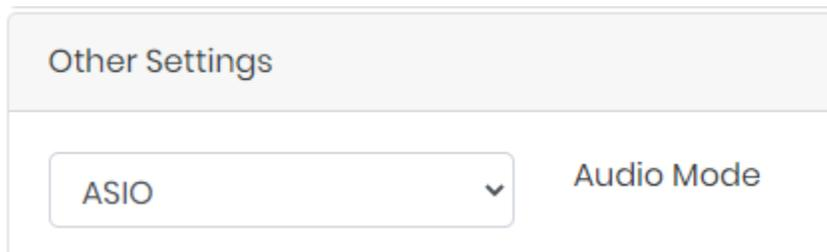
**\*NOTE:** Changing audio modes should only be done when BDS has been bypassed, the audio will stop as the input and output channels are different between audio modes.
